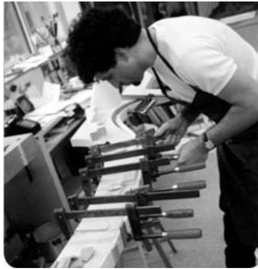
FIGURE 62 Applying the laminated basswood edge strip to the exterior of a stretcher bar. Adhesive is spread between each of the laminates, which are then stacked and held together with jigs (visible in foreground with small clamp). These jigs permit the composite strip to be easily bent around the curves without shifting and to be nailed in place.
