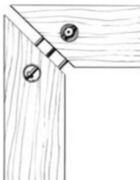
FIGURE 12 c. 1957 James Lebron, New York, NY, expansion bolt stretcher. Not patented.
