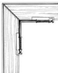
FIGURE 11 Usually redwood members with plates in the miters corners, spring braces in the inner corners, and a metal rod or springs in the cross members.
